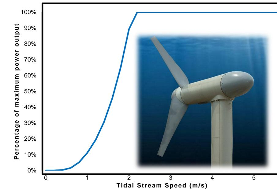
Figure 5: Representative Tidal Turbine and Power Curve ([www.verdantpower.com](http://www.verdantpower.com))
