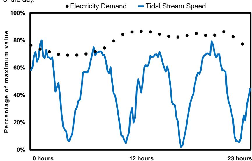
Figure 2: Daily profile of tidal stream speed (prediction based on the derivative of tide height) vs. electricity demand (observed)
