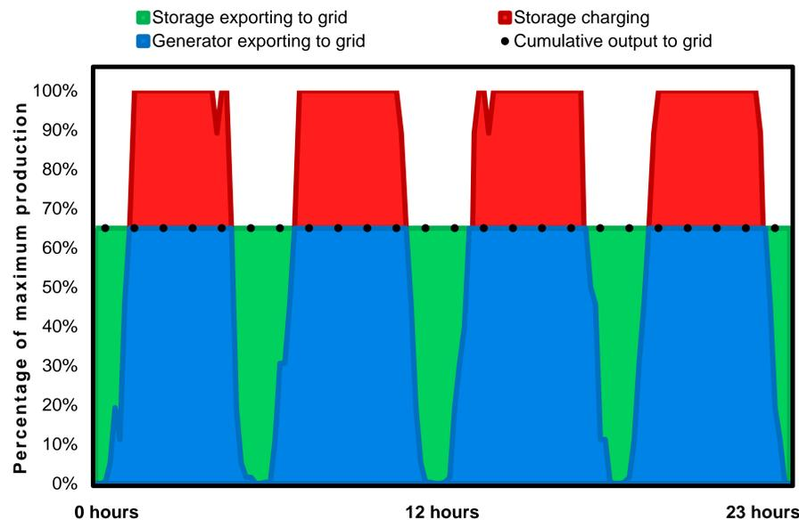
Figure 4: Charge and discharge regime for a typical generator
