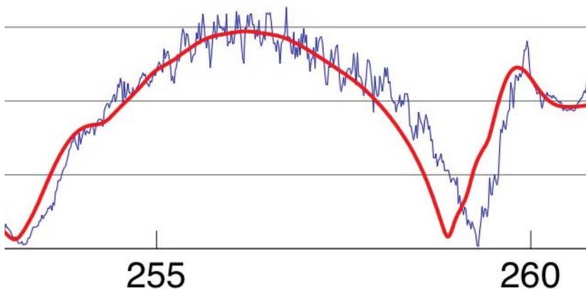
**Figure 1:** A comparison of simulated velocity (red line) and ADCP measurements (blue line) for a location in the Minas Passage. While the simulation can capture the large scale variation, it does not model the high frequency fluctuations.
