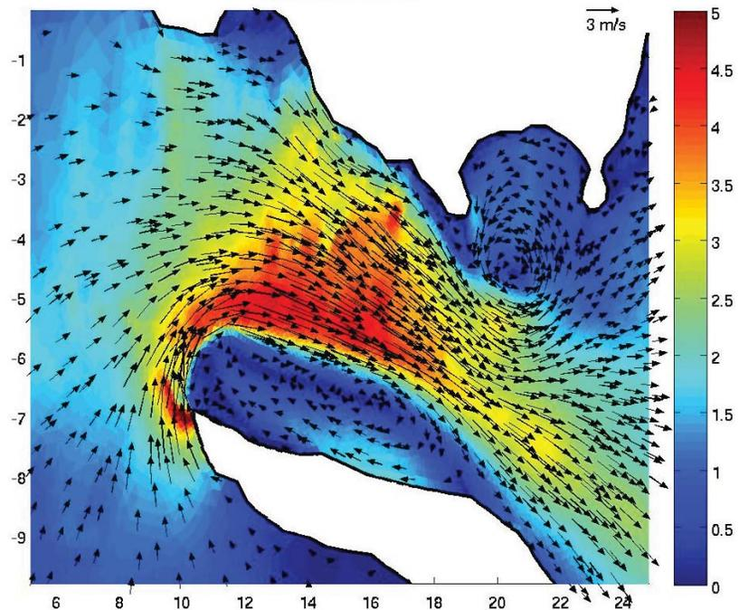
**Figure 2:** A plot of the speed and direction of the flood jet from high resolution 3D simulations of the flow through Minas Passage. Note the asymmetry of the jet and the large eddies north and south of the jet.
