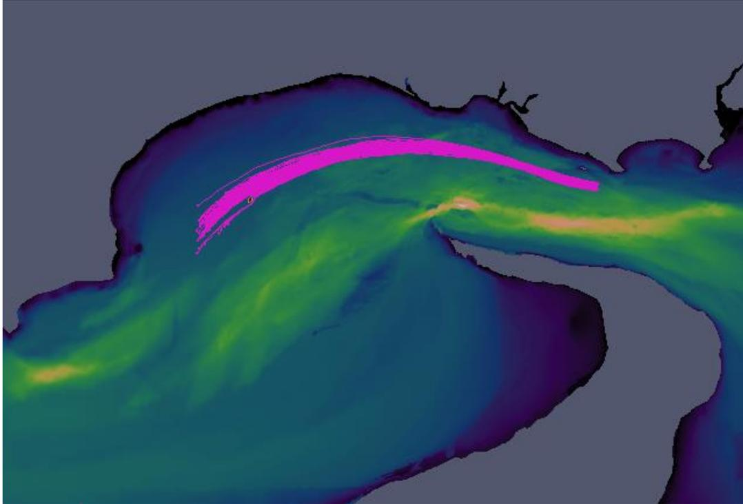
**Figure 1:** A clear wake is shown behind an arbitrary noise source in Minas Passage. The colors represent depth, and the pink trajectories are the particle (fish) path lines, starting from a point near Black Rock.
