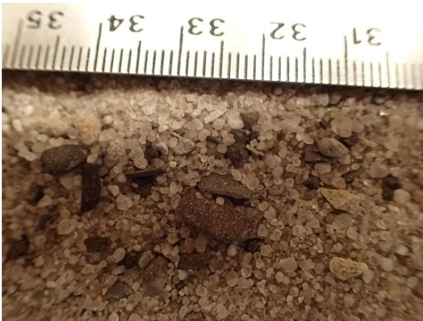
**Figure 2:** Sand comprising the Beaufort formation from the Sirius K-28 well. Mature quartz arenite sand with lithic clasts scattered throughout and woody detritus (fibrous, white). This is the type of sample taken for TCN dating. Image courtesy of Rod Smith, GSC Calgary.
