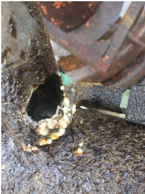
Figure 16 - Examples of corrosion on anodized aluminum housing and connectors with dissimilar metals
