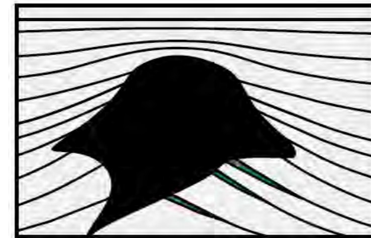
Figure 1.3.27: Schematic cross-sections showing two types of traps against salt in the Gulf of Mexico (from Bouroullec et al, 2017). 2a) Suprasalt: the flank of the diapir and the reservoir have the same dip direction 2b: Infra salt (or subsalt): reservoirs and salt flanks or feeders (or weld feeders) are dipping in the opposite direction. Examples of Gulf of Mexico oil fields are indicated for each style with reservoir types and age; figure number refers to AAPG datashare 81 attached to the oilfield atlas (Weimer et al, 2017)
