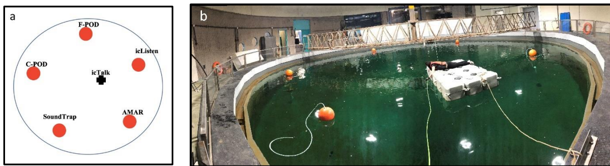
Figure 2: (a) Schematic of the Aquatron Pool Tank showing the placement of PAM instruments and icTalk used for acoustic time synchronization, and (b) photograph of the laboratory based assessment showing the location of surface floats and the floating platform where the icTalk was deployed (photo credit: Tyler Boucher).
