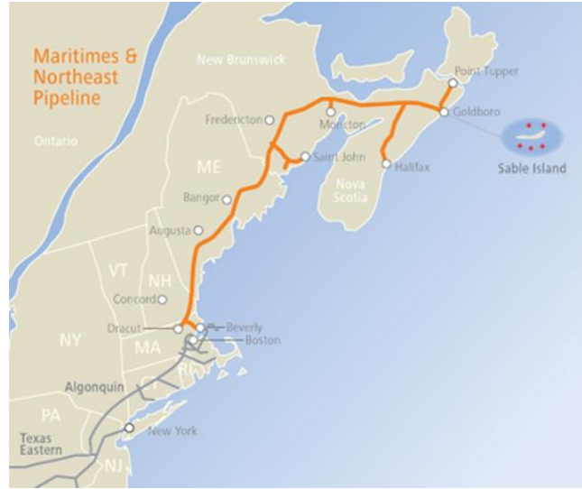
Figure 47 – Maritimes & Northeast Pipeline (M&NP) transmission network map (orange line) 60
