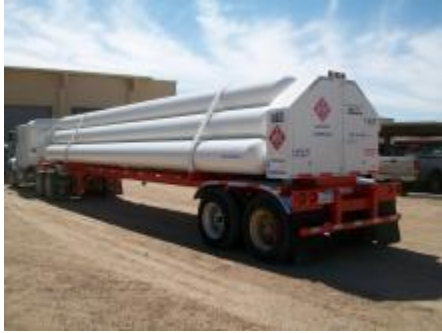
Figure 40 – Compressed H2 tube trailer 52
